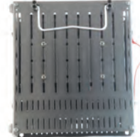
Bottom of TRC-2 showing radio bolted to carrier
