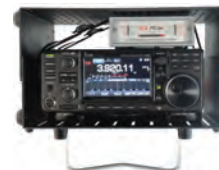
SCS Pactor modem strapped to ICOM IC-7300
