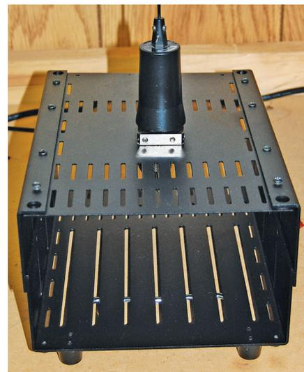
**Figure 18** — The author mounted a 2-meter antenna using another TRC-1 and top cover.
