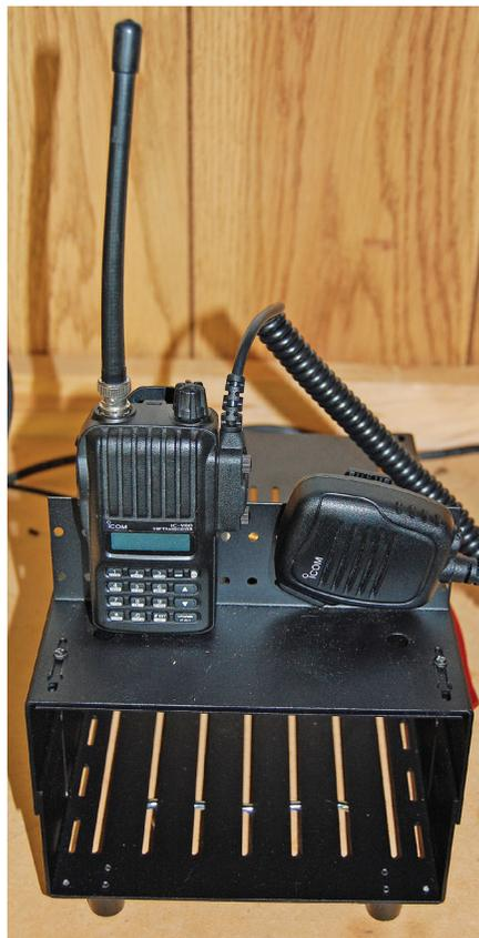
**Figure 17** — The optional HTH-1 bracket can be used to secure handheld radios in an upright position atop the TRC-1. The bracket can also be mounted in the other direction, providing a front cover to protect equipment inside the TRC-1 during transit.
