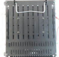
Bottom of TRC-2 showing radio bolted to carrier
