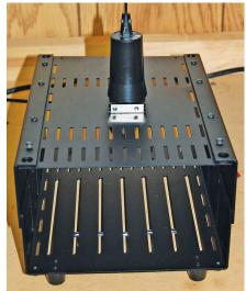
**Figure 18** — The author mounted a 2-meter antenna using another TRC-1 and top cover.
