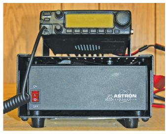
Figure 16 — The author's IC-2200H transceiver and Astron SS-30 power supply mounted on the TRC-1 carrier with optional top cover.
